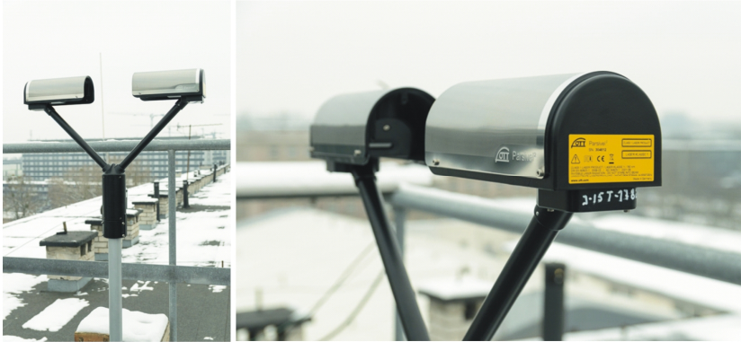
Fig. 1. OTT Parsivel 2 laser disdrometer installed on the observational deck of the roof of the Warsaw University, Institute of Geophysics' building.
