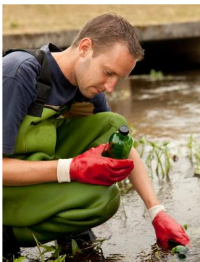
A representative grab sample is used as a primary standard for in vivo phytoplankton measurement
