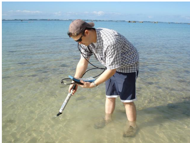
Real-time in vivo phytoplankton measurement using fluorescence sensors on a Hydrolab sonde
