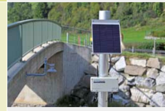
Sensor installation in gauge well or in protective piping at the bank and in the water.
