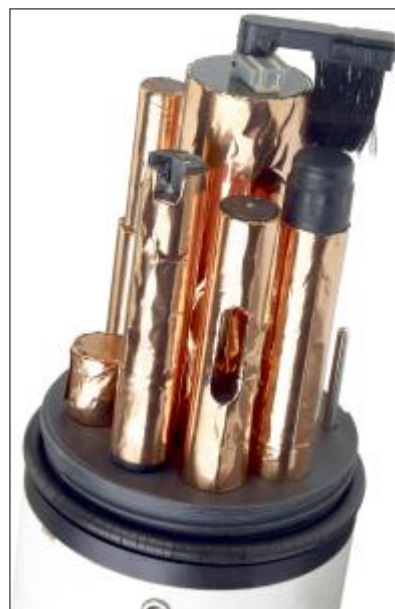
Above: sensors wrapped with copper tape
